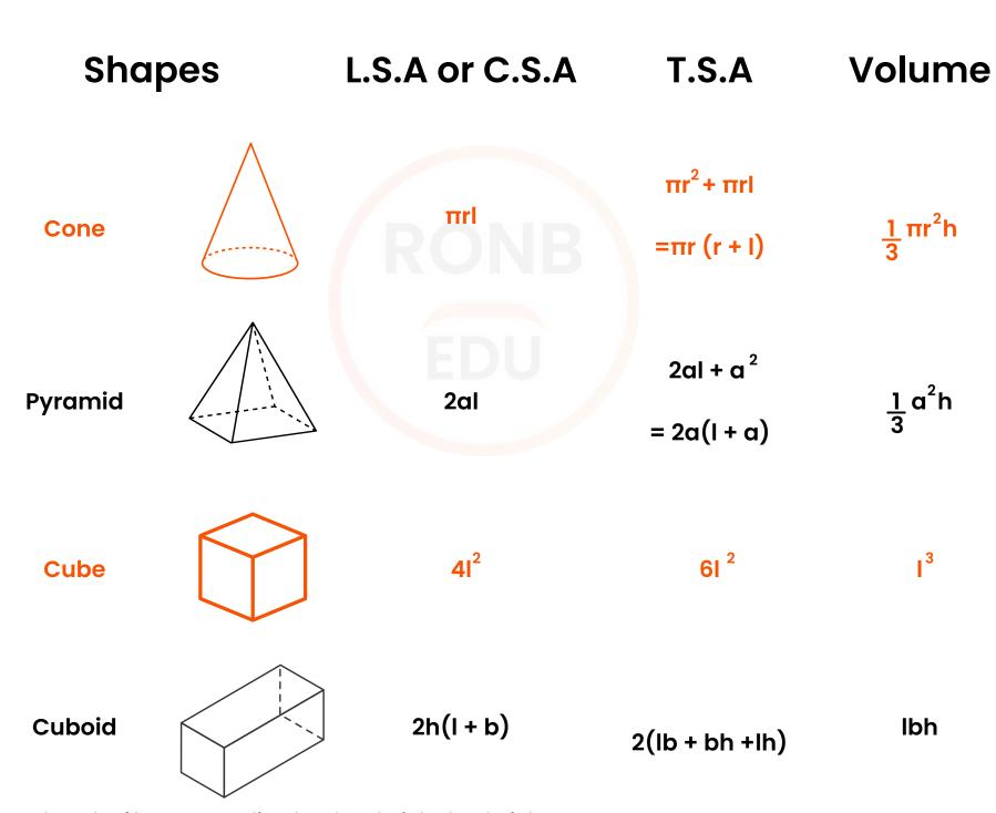
a = length of base, r = radius, l = slant height, h = height Note: CSA is calculated for shapes having a curved surface.
